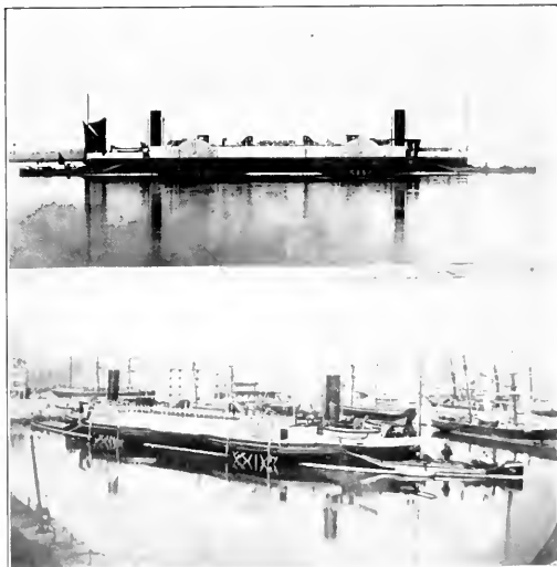
The cross-channel packet Bessemer built in 1875. At the suggestion of Sir Henry Bessemer, her passenger quarters and saloon amidships were suspended on gymbals. In the choppy seas of the English Channel the saloon swung one way and the vessel another, and the passengers in all directions.
